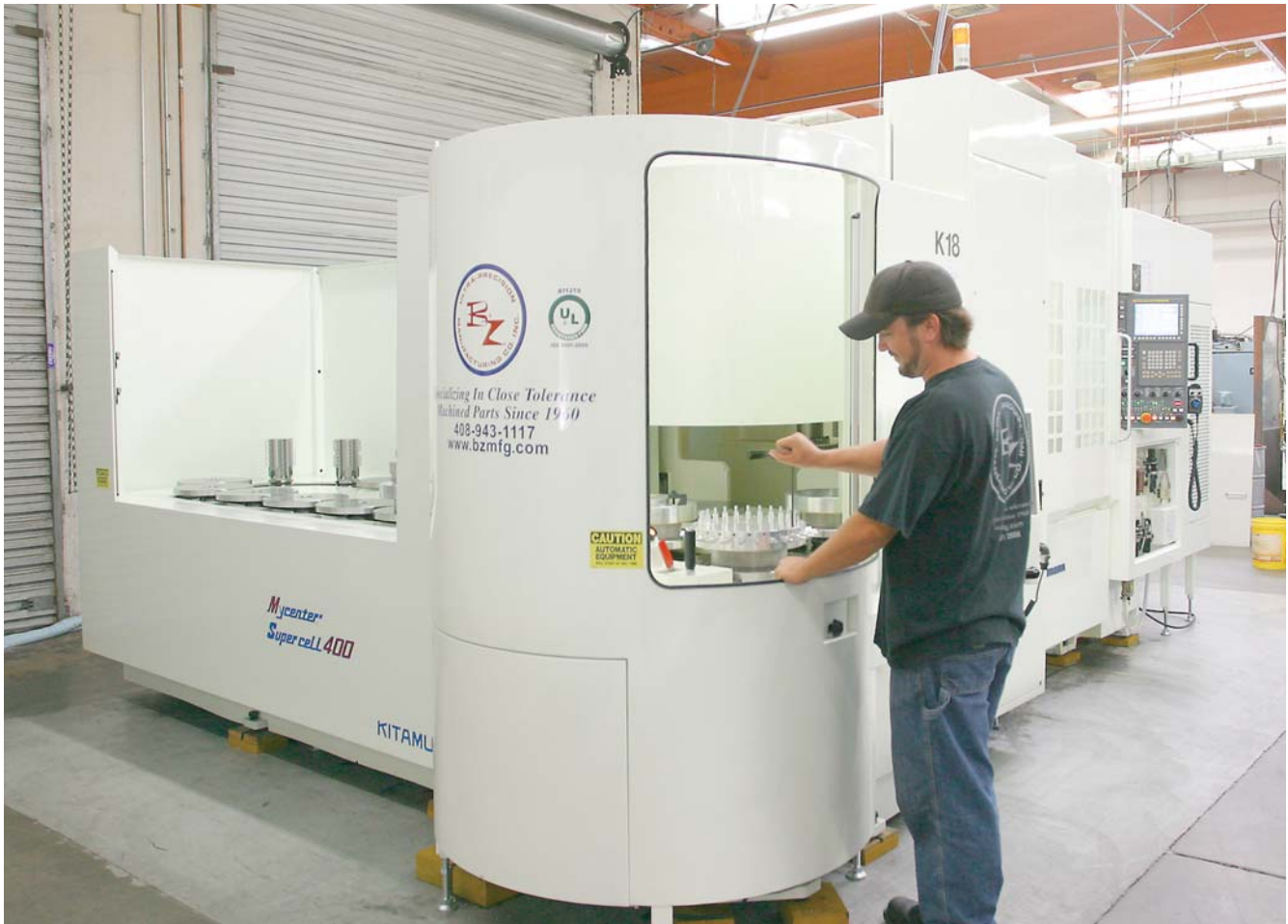
Brian Van Steenwyk, CNC operator, shop foreman at B&Z's 5-axis, 20-pallet Kitamura Mycenter Super cell 400. The machine has a TIVO box on it that permits setting up a week's work in advance. The machine is one of 19 Kitamura's operated by B&Z.
